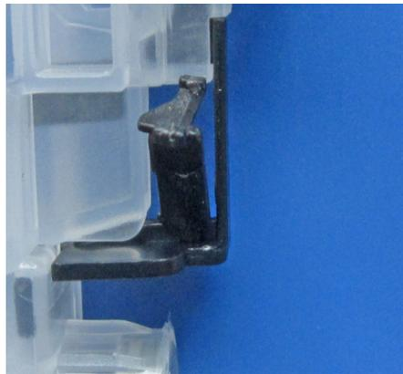
Insert the sensor plate, position it so that the bar on the cartridge fills the groove on the plate.
